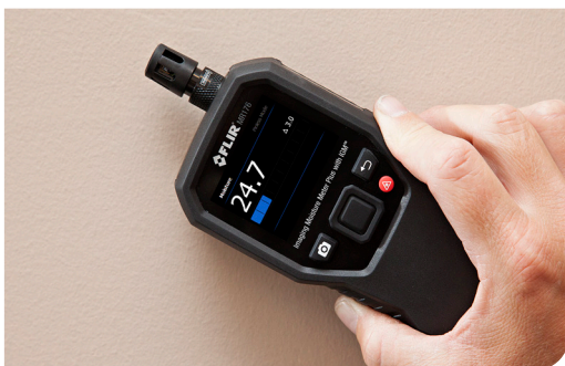
Verify moisture with Pinless measurements
