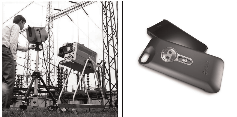
Figure 22.2 LEFT: Thermovision Model 661 from 1969. The camera weighed approximately 25 kg (55 lb.), the oscilloscope 20 kg (44 lb.), and the tripod 15 kg (33 lb.). The operator also needed a 220 VAC generator set, and a 10 L (2.6 US gallon) jar with liquid nitrogen. To the left of the oscilloscope the Polaroid attachment (6 kg/13 lb.) can be seen. RIGHT: FLIR One, which was launched in January 2014, is a slide-on attachment that gives iPhones thermal imaging capabilities. Weight: 90 g (3.2 oz.).
