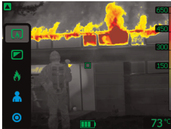
Figure 20.1 NFPA firefighting mode.
